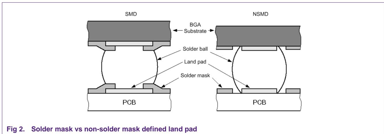
Fig 2. Solder mask vs non-solder mask defined land pad
