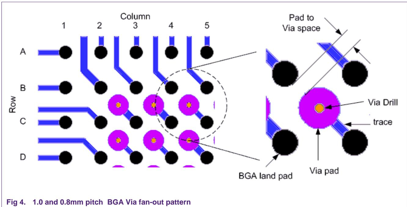
Fig 4. 1.0 and 0.8mm pitch BGA Via fan-out pattern
